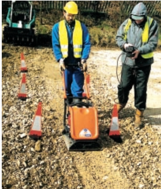
Andy Bell of Errut operates the Errut plate whilst Alan Matthews of AVT records the hand arm vibration figures.
