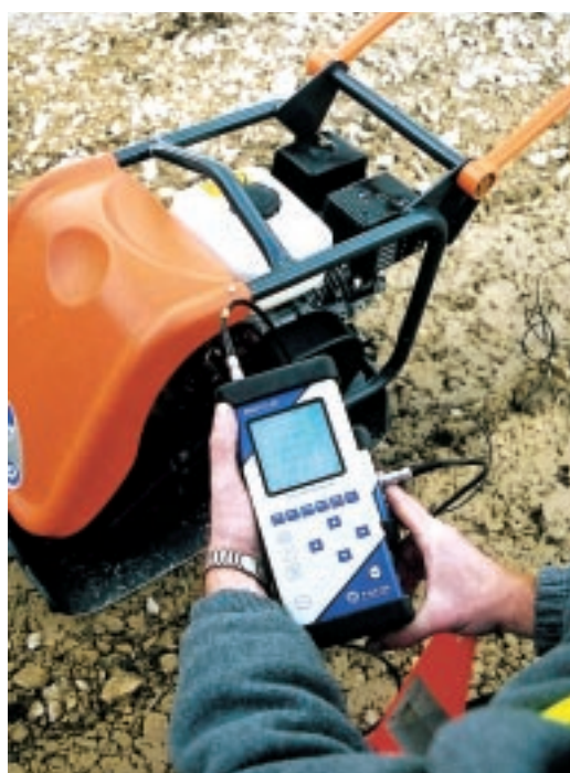
The Svantek instruments were able to measure and record vibrations in three axes simultaneously.
